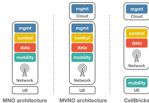
**Figure 1: The network here refers to both RAN and cellular core infrastructure. The Cloud contains those portions of the cellular service typically run in a datacenter (e.g., subscriber database). The MVNO arch. requires in-network support for management because they still rely on usage accounting and authorization implemented in the core.**
