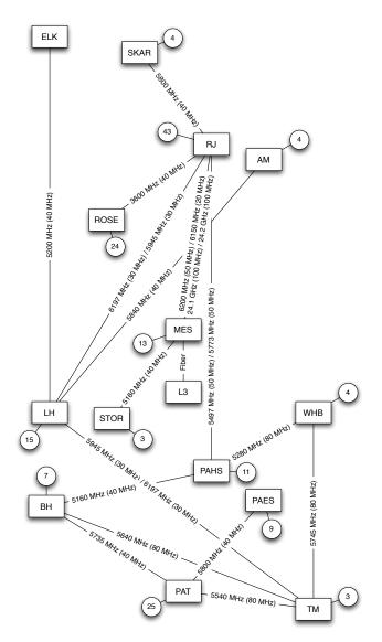
Figure 2: Our WISP network topology as of Q1 2015. Boxes are major sites, labeled by code names. Circles indicate the number of subscribers connected to those sites at that time. Lines depict backhaul links, with frequency and channel width; for full duplex links, we give TX/RX frequencies from South to North.
